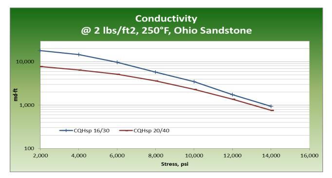
All the above data are typical values obtained according to ISO 13503-2/API RP 19C, and ISO 13503-5. Actual conductivity may vary substantially due to gel damage, fines migration, and other factors.
